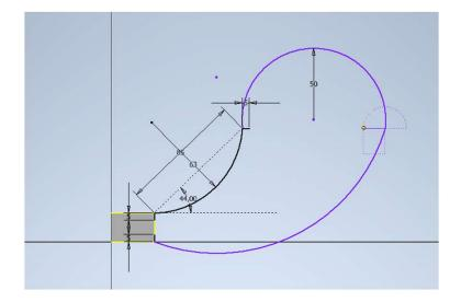
Using the "décalage" tool, shift this shape 5mm inwards.
