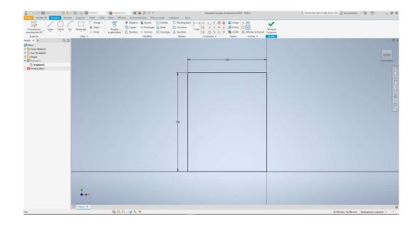
Choose "3d model" from the top bar and select the "extrusion" tool. Then click on the desired face and enter the dimension of 250mm.
