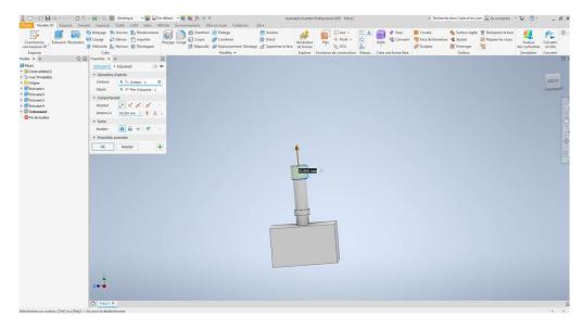
Take the "chamfer" tool and make chamfers on the edges shown in the image.
