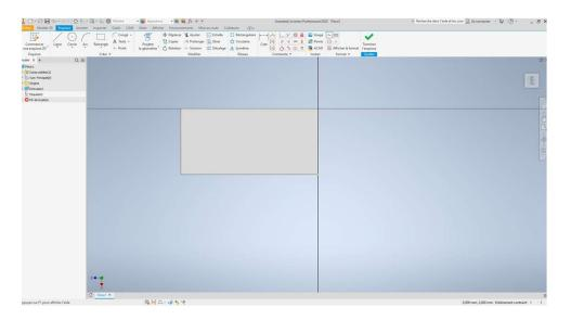
Take the "construction" tool to make the two lines that will give us the centre point of our piece. Then once we have found our center point we need to make a circle of size 50mm.
