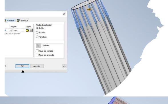
make a chamfer of 0.25 with an angle of 85° and made a leave of 0.2 as on picture
