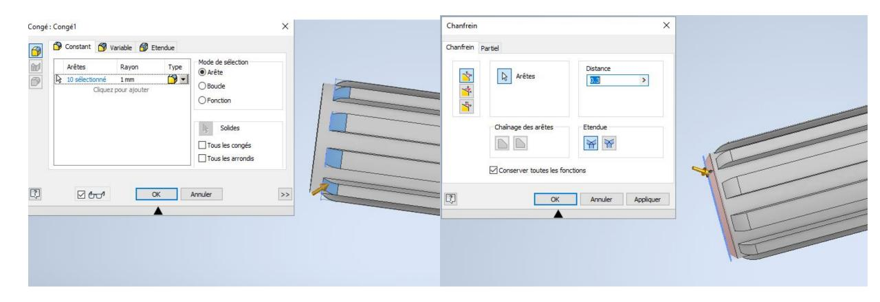
• Make a 1mm fillet at the bottom as shown and make a 0.3 chamfer at the bottom
