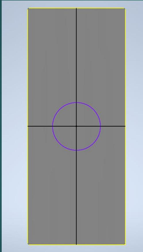
12 : create an Esquisse on the top of a rectangle and recreate the drawing here by using the tools : "Ligne" et "Cercle"
