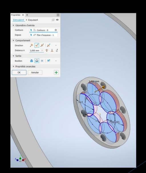
Step 10:Add geometry formsAnd repeat it withThe circular grid
